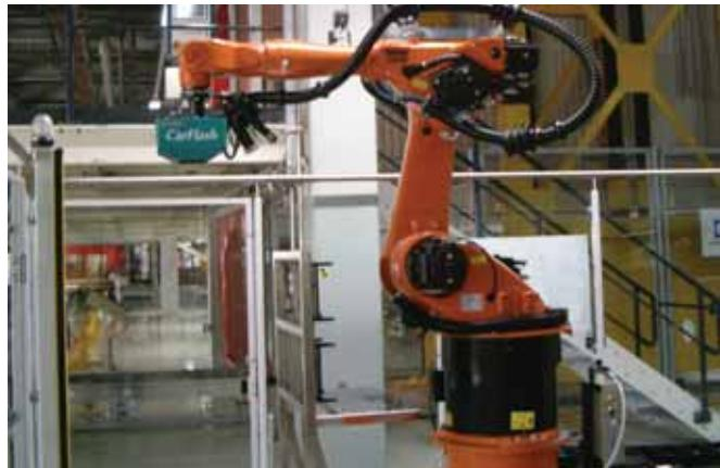
***In the case of robotic multi-layer ultrasonic thickness gauging, measurements are obtained by the use of non-contacting position sensors and a special contacting ultrasonic sensor.***
